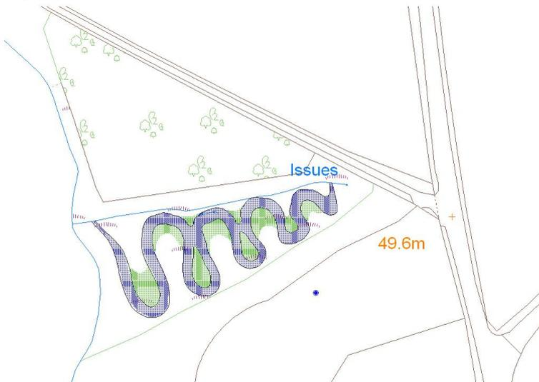
Create a meandering channel which overflows during high flows. Plant with mixed aquatic plants.
