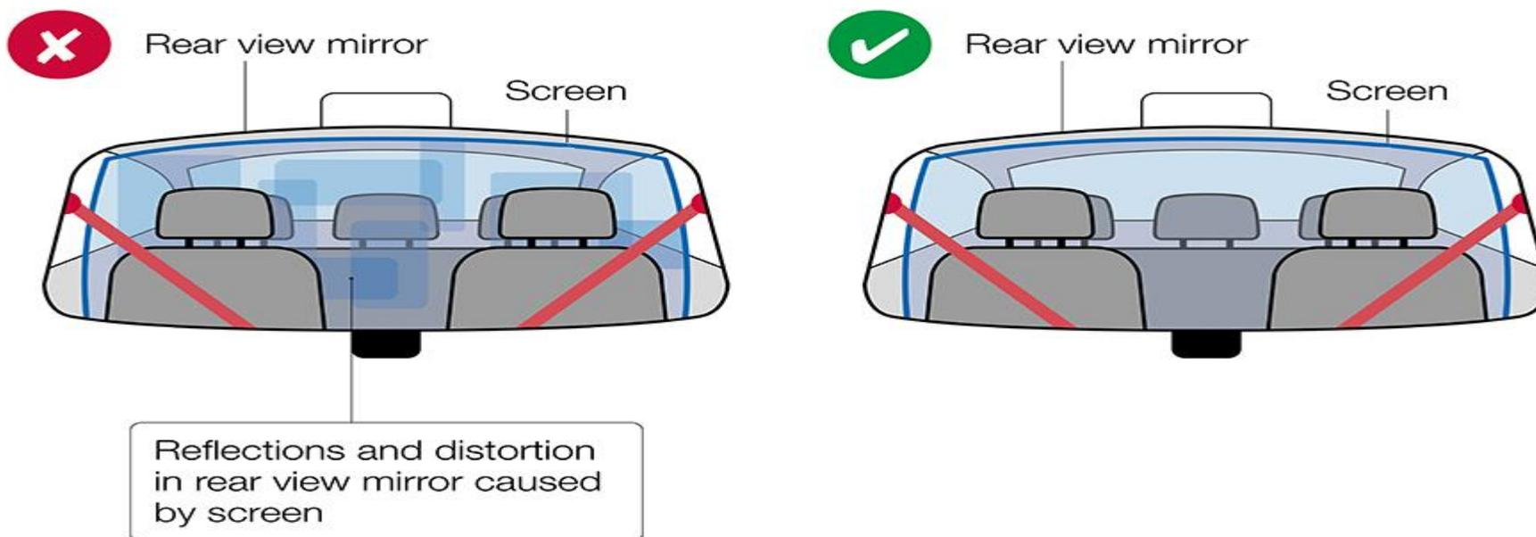
Ensure that any fittings to the vehicle do not compromise the safety and electrical systems on the vehicle. Hybrid and plug-in hybrid vehicles will have high voltage cables that may be hidden. Do not drill holes or make fixings to vehicle trim if you do not know what is behind a panel. Screens must be fitted so that they do not interfere with the operation of seats and head restraints as shown in figures 3a and 3b.
