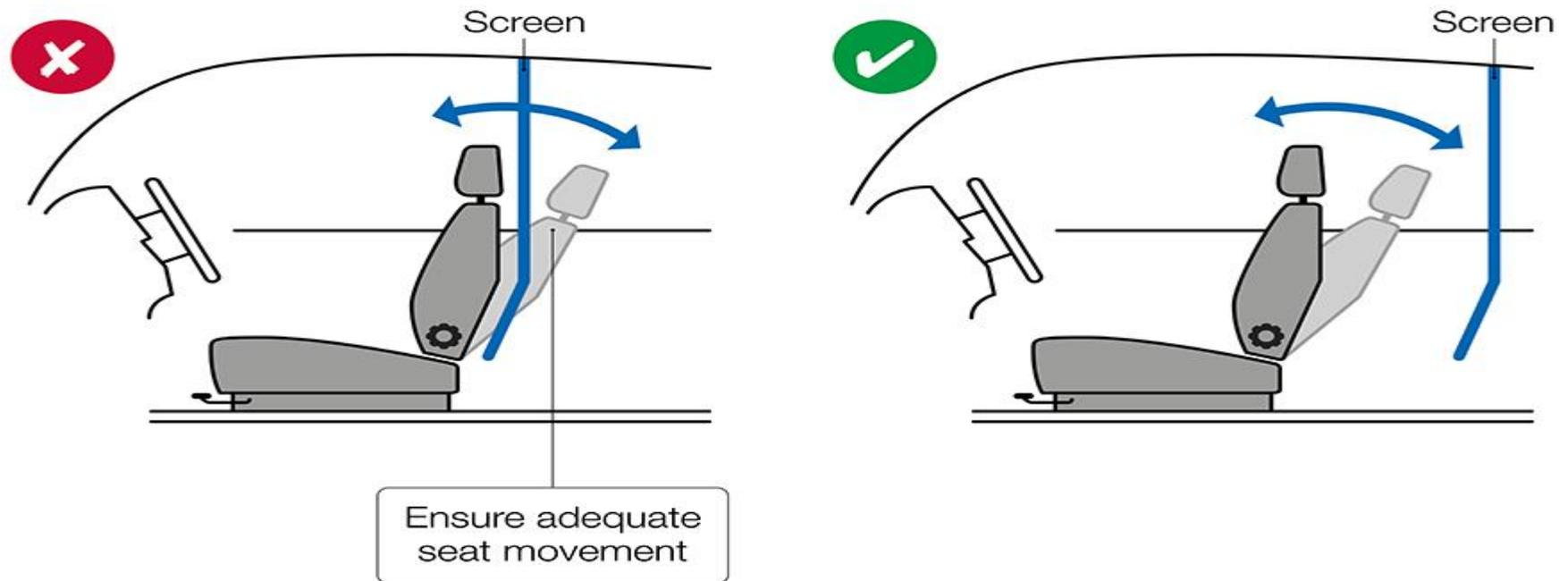
The fitting of the screen must not prevent the correct operation of seatbelts. The seatbelt webbing should not chafe against the screen or the fixing points, or adversely affect the operation of seatbelt pretensioners.
