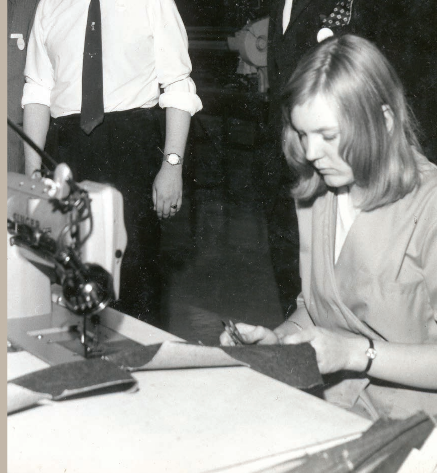
Sewing back-pockets on a hemming machine at Levi's, c. 1970.
