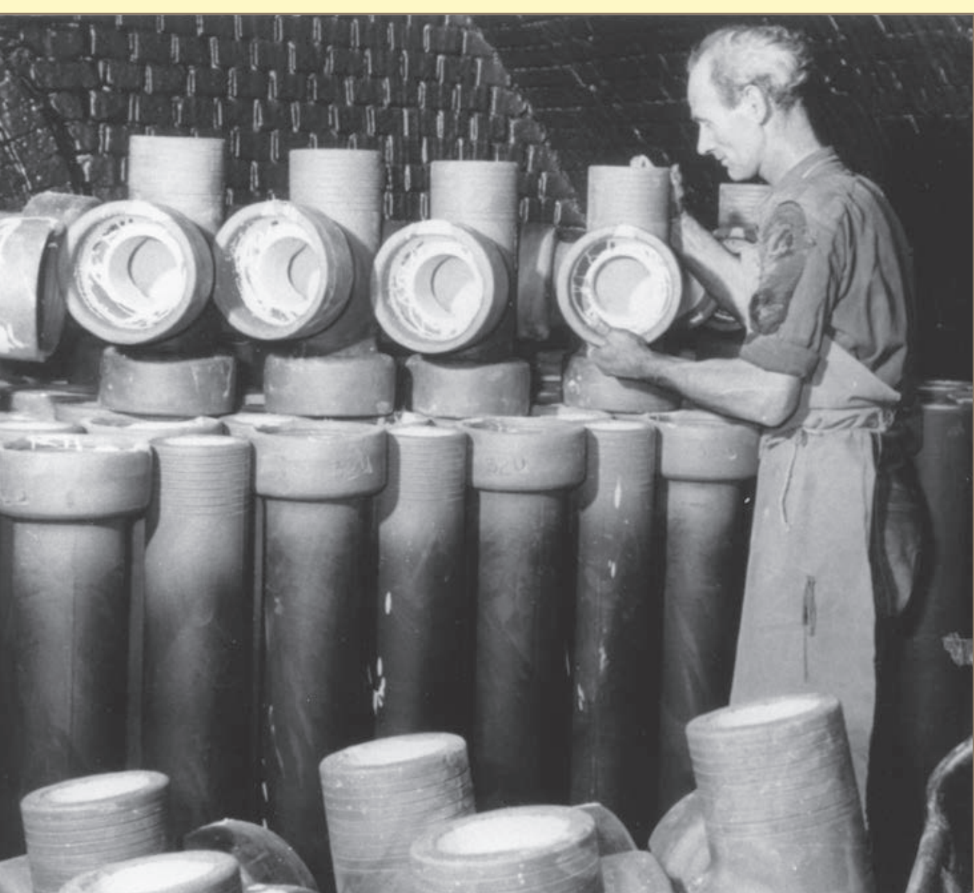
Stacking fireclay pipes in the kiln at Bathville Pipeworks, Armadale. The fireclay seams in central Scotland were used to make bricks, pipes, chimney cans and sanitary ware. Both men and women were employed in the fireclay industry.
